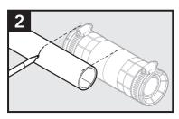
Align both ducts at the center of the coupler and mark ends.
