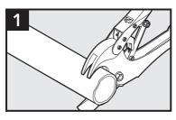
Cut conduit flush with duct cutters.
