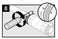
Verify the band clamp is positioned in the groove and fully tighten it down with a 5/16" nut driver. Never use a drill to tighten clamp.
