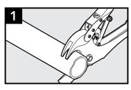
Cut conduit flush with duct cutters.
