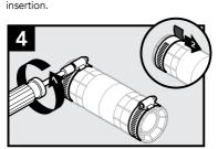
Loosen band clamps and move them towards the middle of the coupler. Lightly tighten to hold in place during conduit insertion. (continued)
