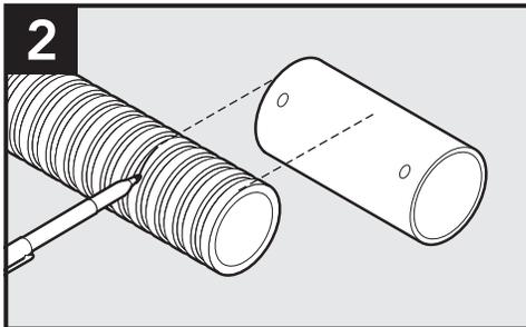
Overlap ends of conduit. Place duct at center of coupler and mark at the end.
