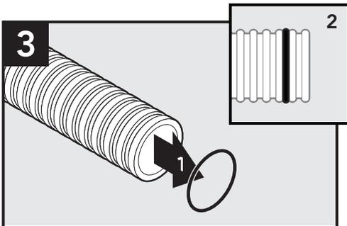
Take one duct and install O-ring gasket. The interior of the O-ring has a high profile that snaps into place. Ensure it is seated in the second corrugation.
