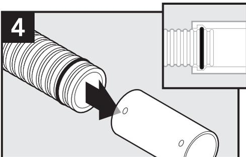
Insert the gasketed end of the conduit into coupler. The lock ring on the inside surface of the coupler should snap into a matching corrugation. A light coating of water-based lubricant can be used to aid in installation.
