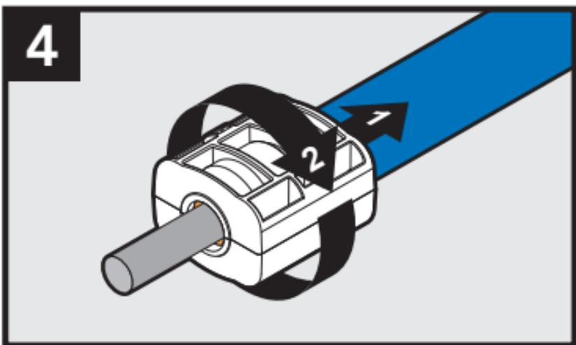
Turn connector while pushing towards the duct.
