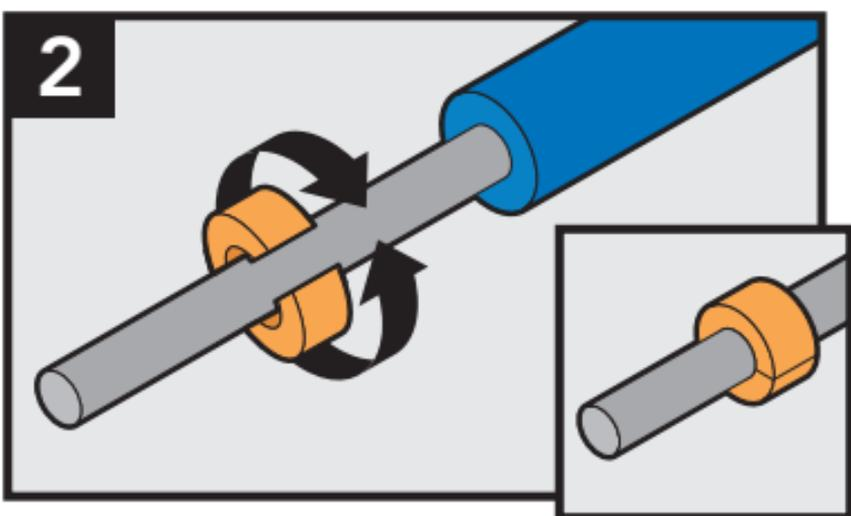
Select required seal and install on cable.
