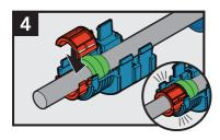
Connect both red pieces around the cable, against the flat side of the seal. The red pieces will extend past the bottom of the blue cover piece.
