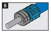
Tighten the nut manually to close the gap around the cable. **DO NOT** use tools.
