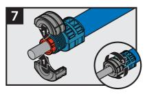
Close both black pieces around the cable and tighten the nut only until touching the red pieces. **DO NOT** over tighten.
