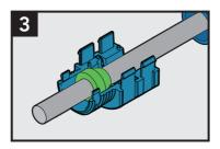
Place seal around the cable and position seal inside one of the blue cover pieces.
