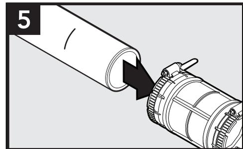
Push conduit into the coupler past the grip ring and O-ring until it hits the center stop and the mark is aligned with the end of the coupler. This ensures the O-ring is seated properly.
