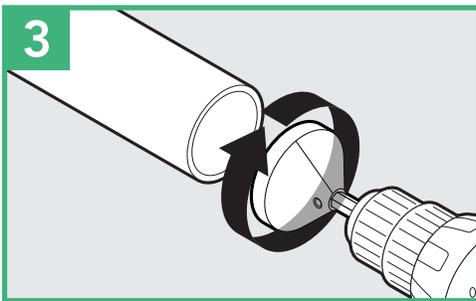
Chamfer the leading edge of the conduit for smoother insertion.
