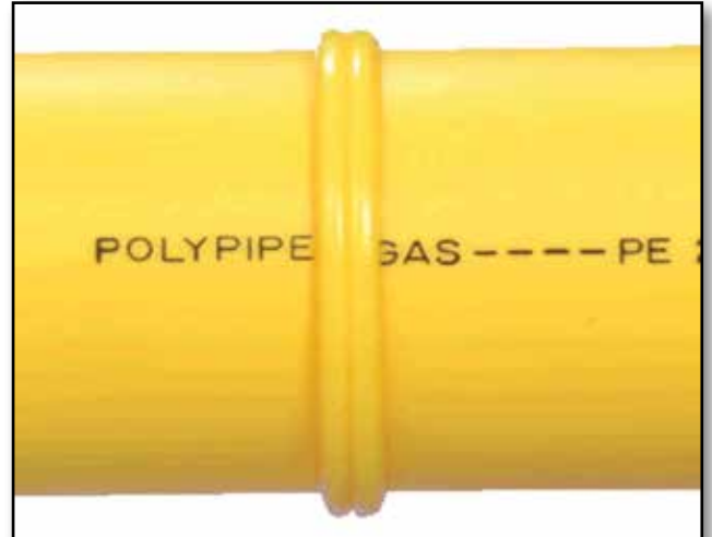
Melt bead too large due to excessive heating and/or overpressurization of joint
