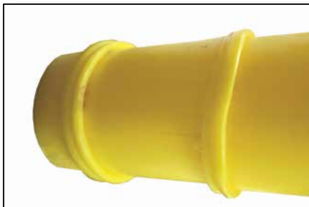
Pressure fluctuation, misalignment over pressurization
