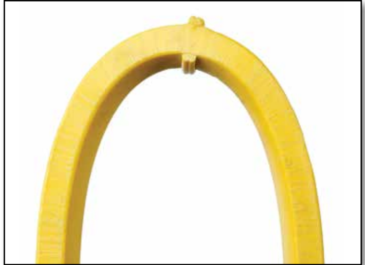
BEND BACK TESTING - NO GAPS OR VOIDS
