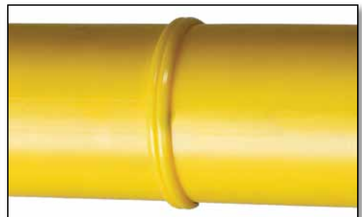
PROPER ALIGNMENT AND DOUBLE ROLL-BACK BEAD
