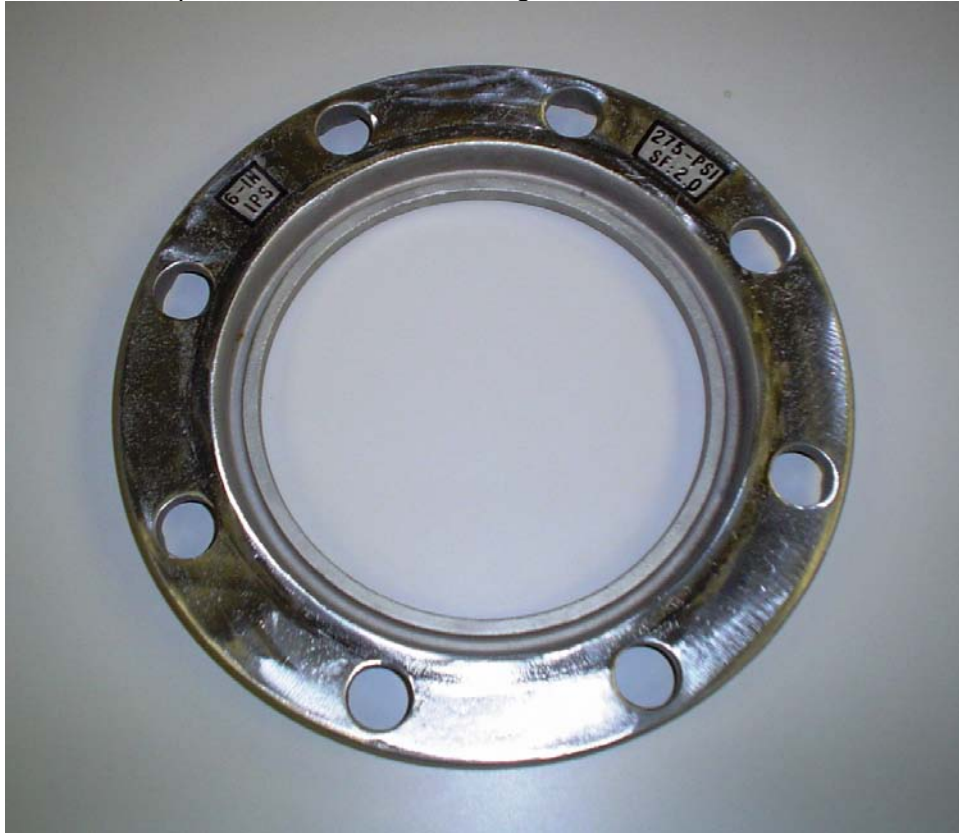
Figure 4 Cast Stainless Steel, Lap-Joint Flange, 6-inch IPS
