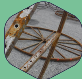
L-Bracket Flange with Punch-out Holes
