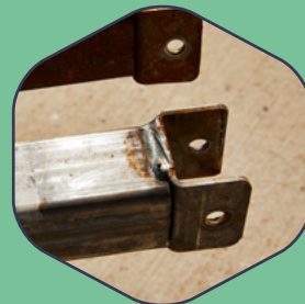
Exposed Bead Welding Not Acceptable
